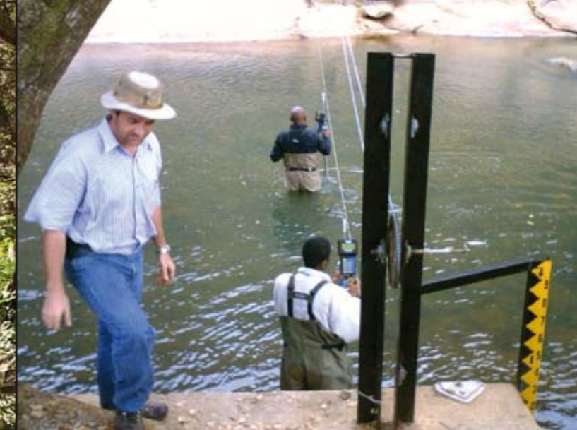
River flow measurement using an Acoustic Doppler Velocimeter in the Crocodile River, South Africa (Photo D. Joubert, Hydrology Mpumalanga, 2005)
